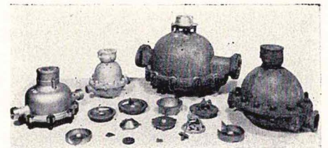
Various water meters and parts cleaned in the American Suction Air Blast Cabinet.
